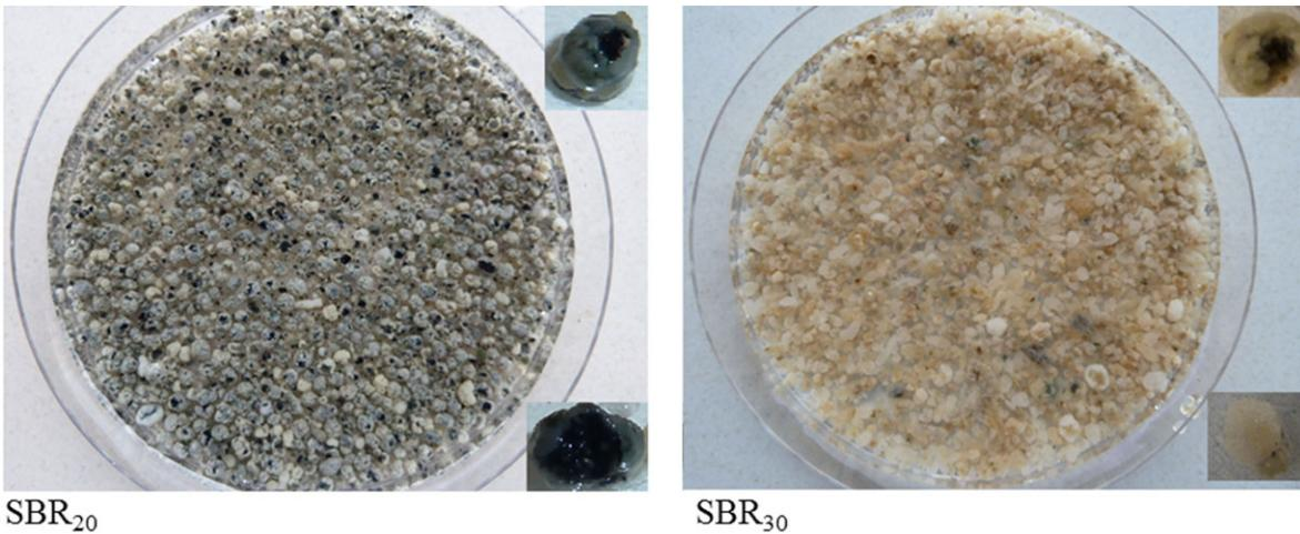
**Figure 3.** Granules from SBR<sub>20</sub> and SBR<sub>30</sub> during operation in Phase II. The core of big granules is shown in detail in the right side of each picture. [Color figure can be seen in the online version of this article, available at <http://wileyonlinelibrary.com/bit>]
