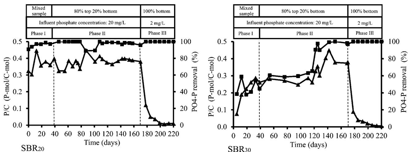
**Figure 1.** Phosphorus (P)-release/COD uptake ratio (▲) and P-removal (■) in the long-term operation of the SBR<sub>20</sub> (a) and SBR<sub>30</sub> (b). Removal of excess sludge for controlling SRT was performed in three different ways: mixed sample during aeration (Phase I), 80% from top and 20% from bottom of the sludge bed (Phase II), and 100% from bottom (Phase III). P-influent concentration was 20 mgP/L in the first two experimental phases and 2 mgP/L in the last phase.
